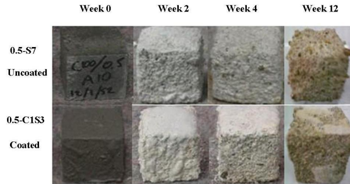
Figure 9: The deterioration of uncoated specimen (Top) and specimen coated at the age of 1 day (Bottom) with cement-only w/b 0.5 during submersion period
