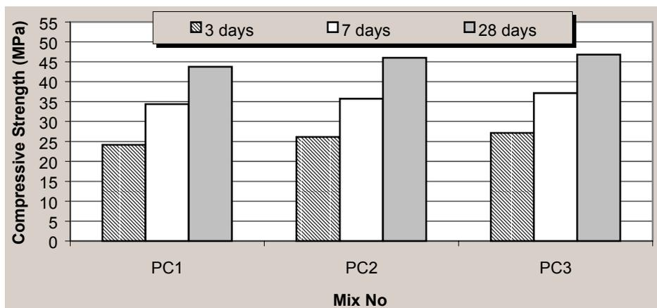
Fig 1. Compressive Strength of Type-GP concretes
