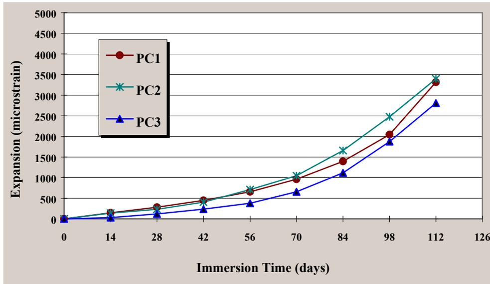
Fig. 6 Length Changes of Samples in Sulphate Solution for Type-GP Concretes
