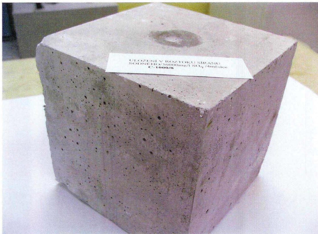
Stored in SO 4 solution 36000mg/l 4 months Sample 8 with C-1000
