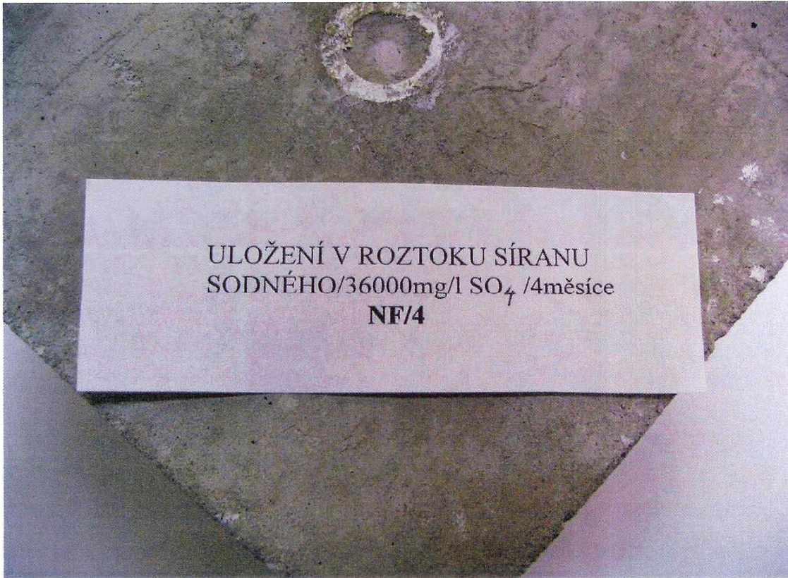
Stored in SO 4 solution 36000mg/l 4 month Sample 4 with NF
