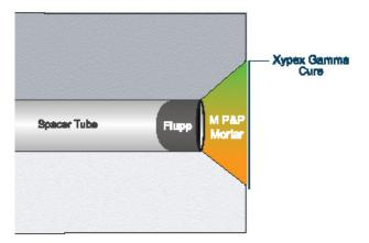
Application schematic and photos illustrating use of the repair system.
